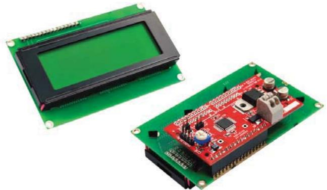
*Serial LCD II with 2x20 characters LCD display module.*
