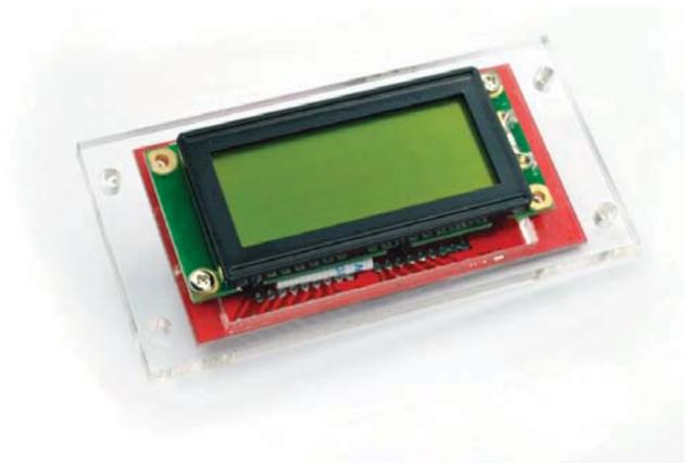
*Serial LCD II with 4x20 characters compact LCD display module. Available as an option is a acrylic mounting bracket.*
